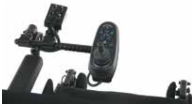
Centre mount joystick with actuator box
